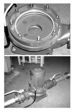
4) Replace the gasket/O-ring of the housing.
