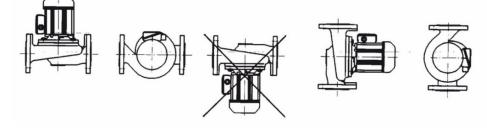
The heavier pumps should be fastened to a foundation of concrete which is isolated from the floor f.ex. with 20 mm thick gum or cork plate(s). The weight of the concrete foundation must be about 1.5 times the weight of the pump.
