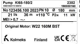
Manufacturing year and month Component number Impeller diameter and material Nominal power of motor
