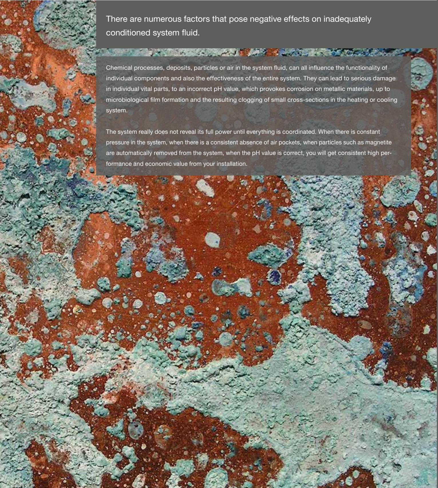
There are numerous factors that pose negative effects on inadequately conditioned system fluid.
