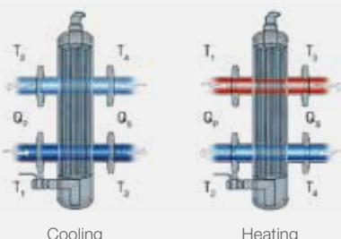
Situation 2:  $Q_p < Q_s$   $\Delta T_p > \Delta T_s$   $T_2 = T_4$
